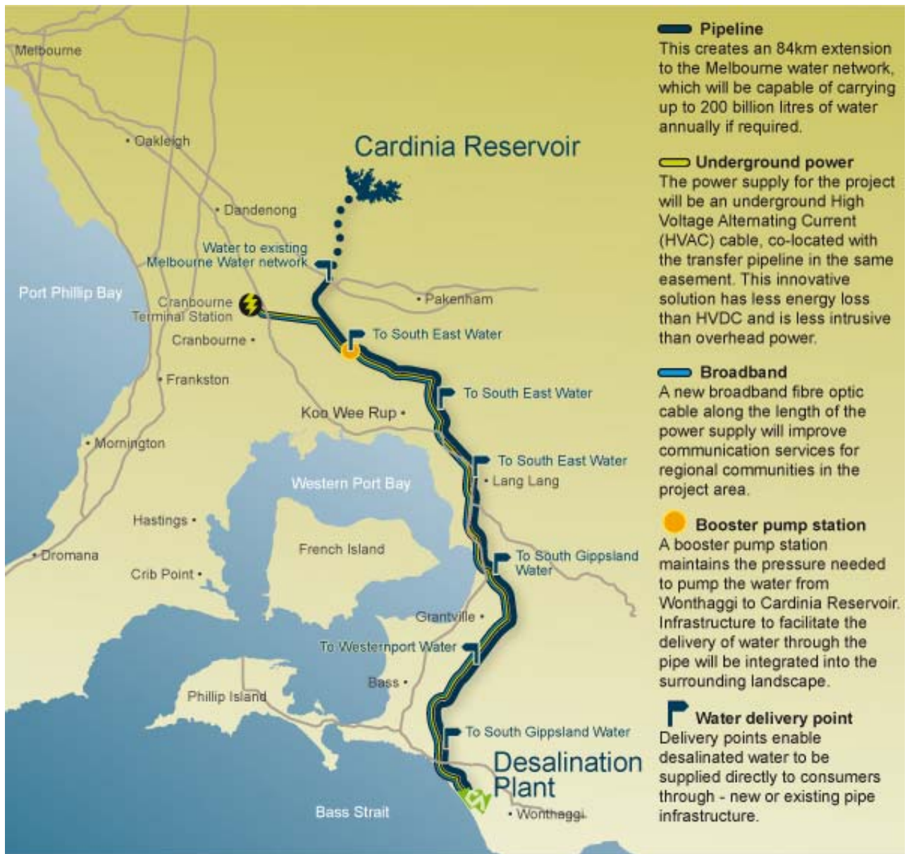
Figure 4.4 – Wonthaggi Desalination Plant Underground 220kV Cable Route
